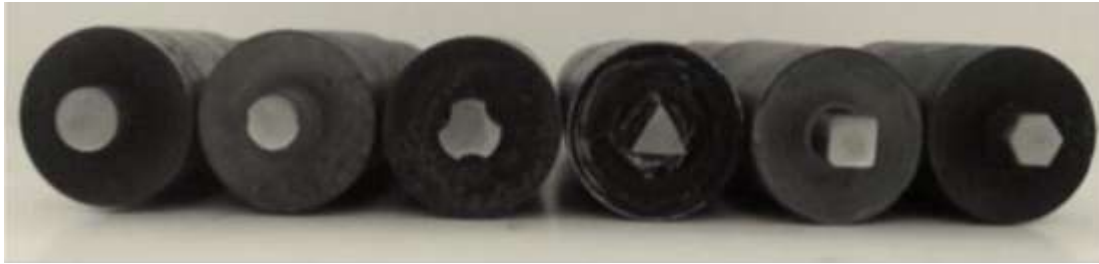
Figure-3:- Geometric shapes of FSP/W tool: a) Cylindrical b) Threaded c) Triflute d) Triangular e) Square f) Hexagon [14]
