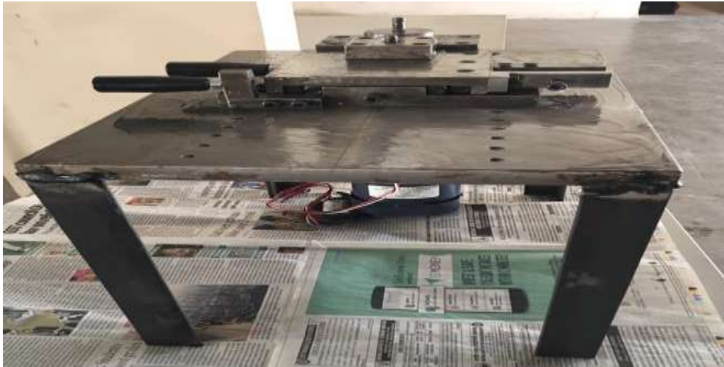
Fig: Computerised Gear Roll Tester(Assembly)
