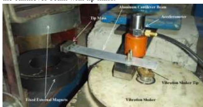
Fig.5 Cantilever beam with tip mass in magnetic field
