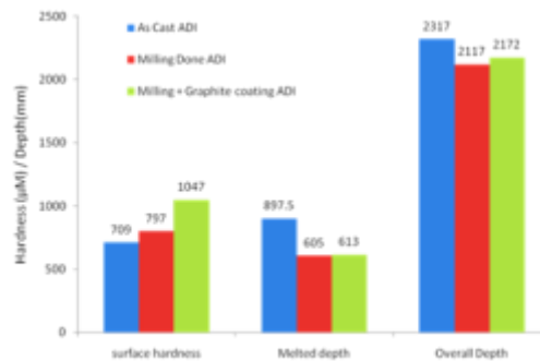
Fig.6. Effect of surface conditions on surface hardness, melted depth and overall depth of ADI
