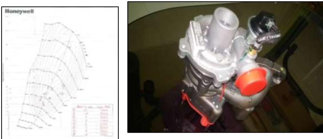
Fig-1: Compressor map and acquired Turbocharger from Honeywell
