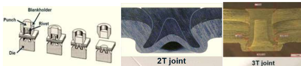
Fig 2. Self-Piercing Rivet applied on Range Rover Sport
