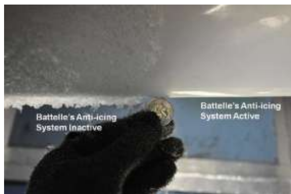
Fig-3: The RNS technology employed by Battelle on a wing section exposed to icing conditions. The wing's right-hand side is ice-free following the usage of Battelle's anti-icing system [1].
