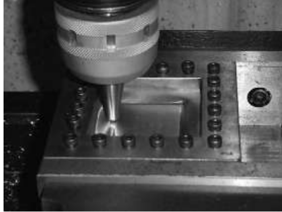
Fig. 5 Incremental forming of an aluminium sheet on CNC milling machine [3]
