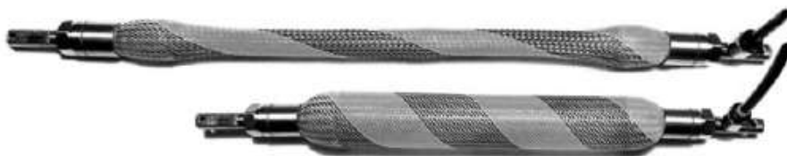
Fig-1: Extended and contracted air muscle [5]
