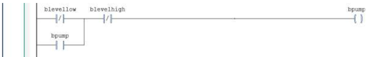
Fig-3 Ladder Diagram PLC Programme for Water Level Control
