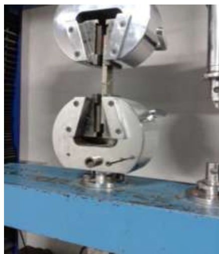
Fig.3 Schematics of the experimental setup for Measuring the strains and the joint strengths
