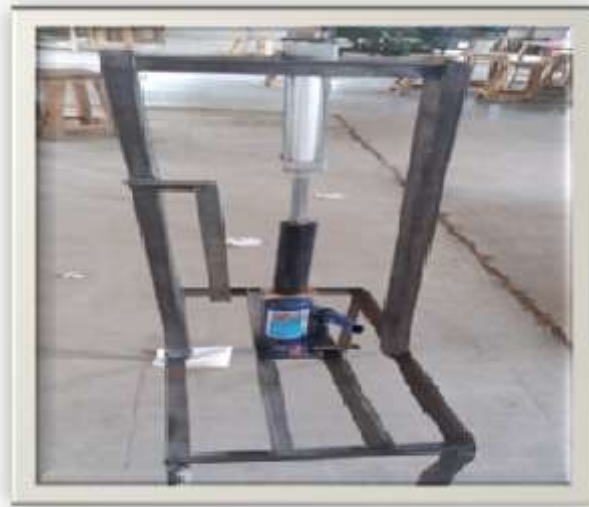
Fig.1 Hydraulic spring stiffness testing machine
