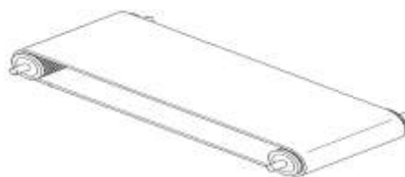
Fig.5 Flat Belt Mounted on Shaft
