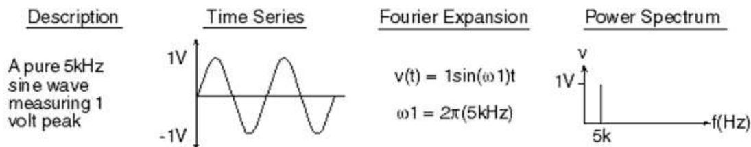
Fig.4 Transformation from Time Domain to Frequency Domain
