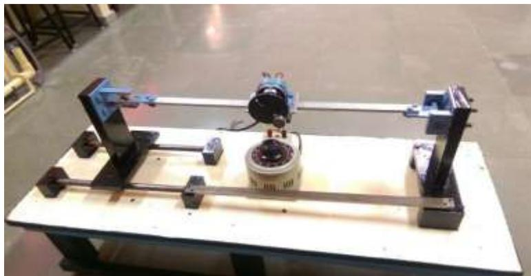
**Fig.2 Vibration Test Rig Prepared by Nikhil T. et al [1]**
