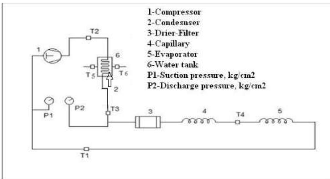
Figure 4: Schematic diagram
