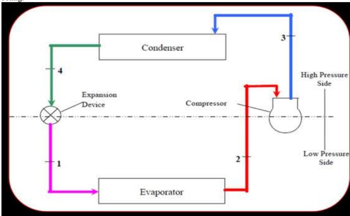
Figure 1: Vapour compression system
