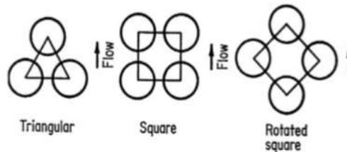
**Fig. no. 2: Tube arrangement in shell and tube heat exchangers**
