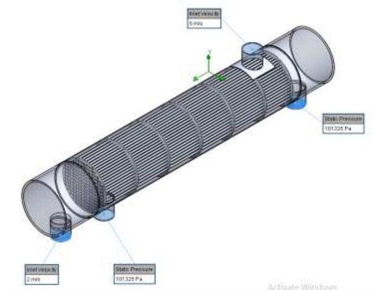
Fig. No. 6: Applying boundary conditions
