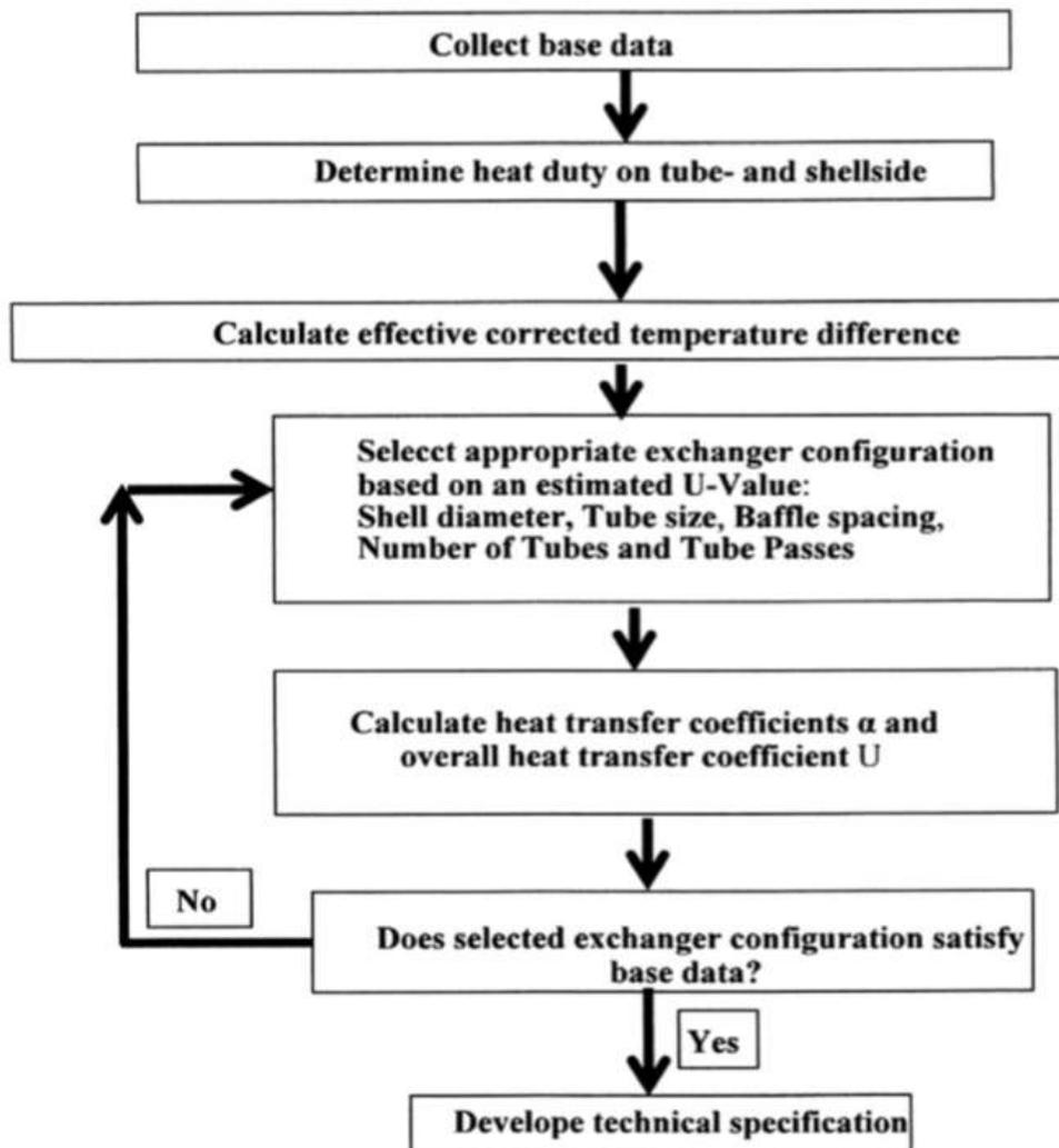
Fig. no 1 Procedure flowchart for thermal design of Heat Exchanger
