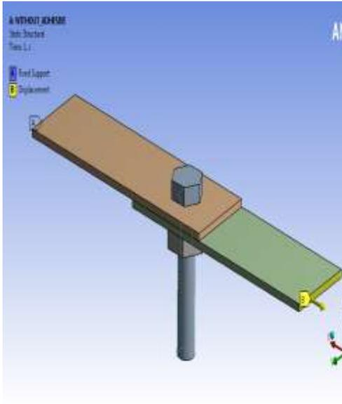
Fig.7 Constraint for bolted joint
