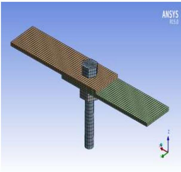
Fig.5 Mesh Generation in bolted joint
