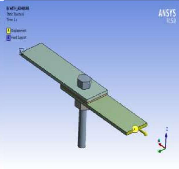
Fig. 8 Constraint for Hybrid joint
