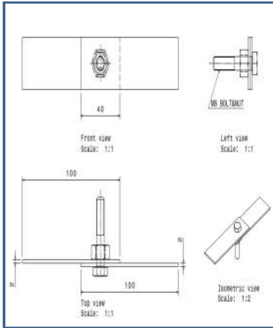
Fig.3 Drafting of bolted joint
