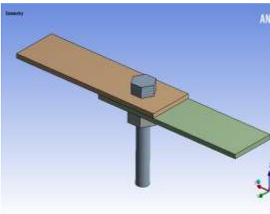
Fig.1 CAD Model of bolted joint
