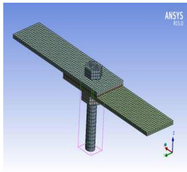
Fig.6 Mesh Generation in Hybrid joint
