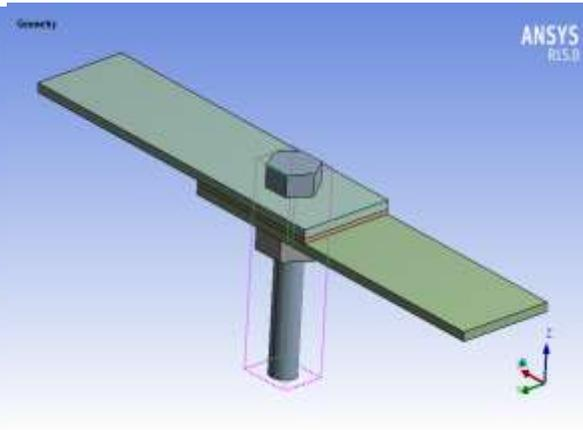
Fig.2 CAD Model of Hybrid joint
