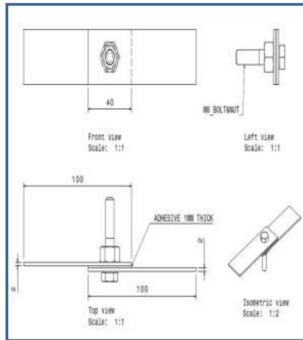
Fig.4 Drafting of Hybrid joint
