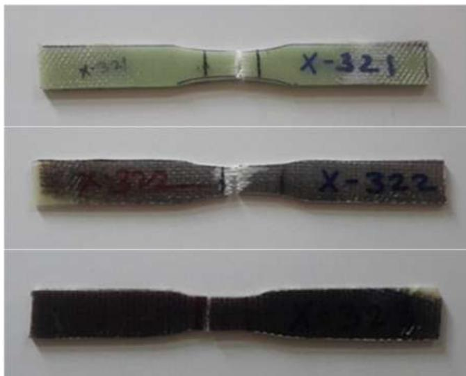
**Fig-1: Tensile test specimens after testing**
