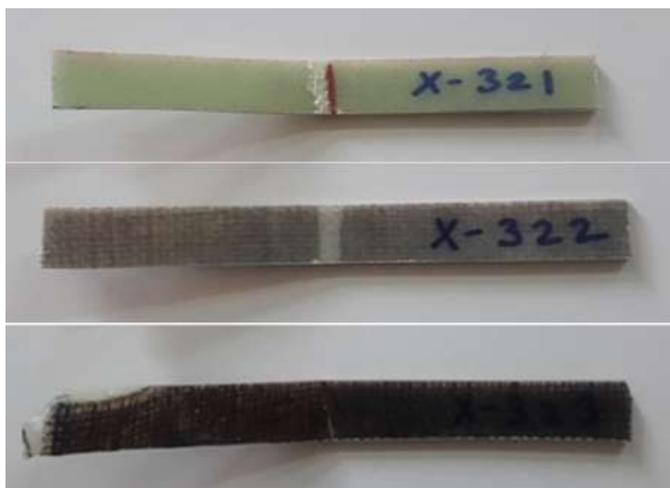
Fig-3: Flexural test specimens after testing
