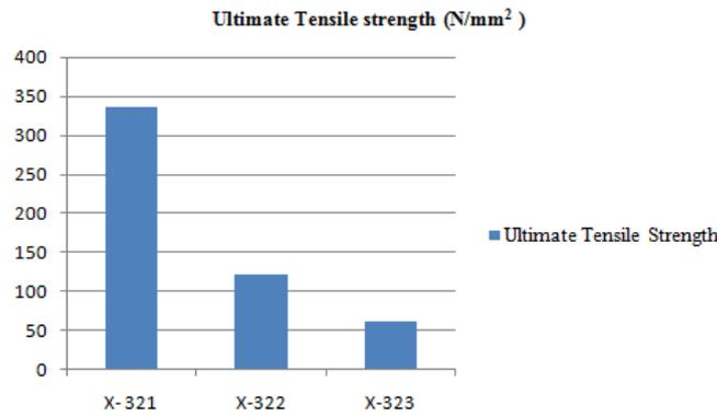
Fig-4: Variation in Ultimate Tensile Strength
