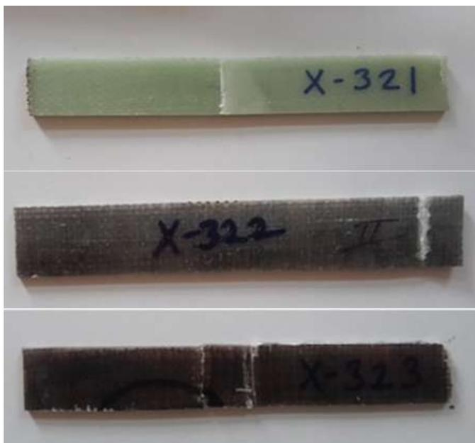
**Fig-2: Compression test specimens after testing**
