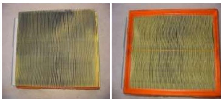
Fig.3.10 Engine Air Filter Clean and Dirty Side
