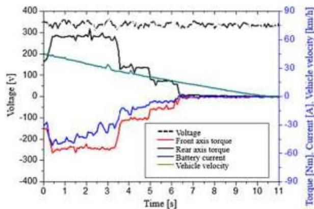
Fig-4: Test results of serial 2 regenerative braking strategy
