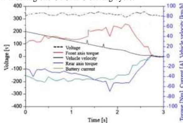
**Fig-2: Test results of parallel regenerative braking strategy.**
