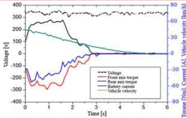
Fig-3: Test results of serial 1 regenerative braking strategy.
