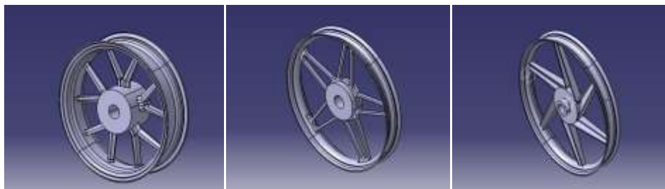
Fig-3: Modelled Rims CATIA V5
