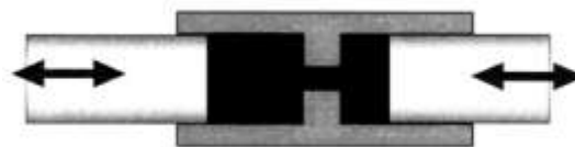
Fig 5. Reciprocating extrusion compression
