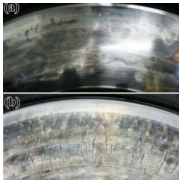
Fig-3: Presence of hot spot and thermal cracks on the disc surface [2]
