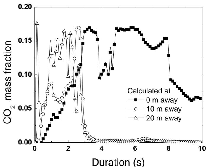
Figure 12 CO<sub>2</sub> mass fraction calculated in Z direction (0, 10 and 20 m away)
