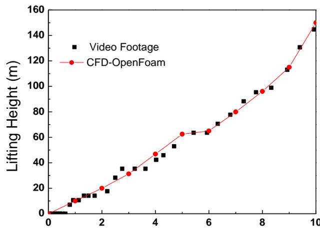
Figure 9: Comparison of lifting height of fireball using video footage and CFD simulation
