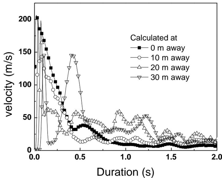
Figure 18: Calculated velocity in Z direction (0, 10, 20 and 30m)
