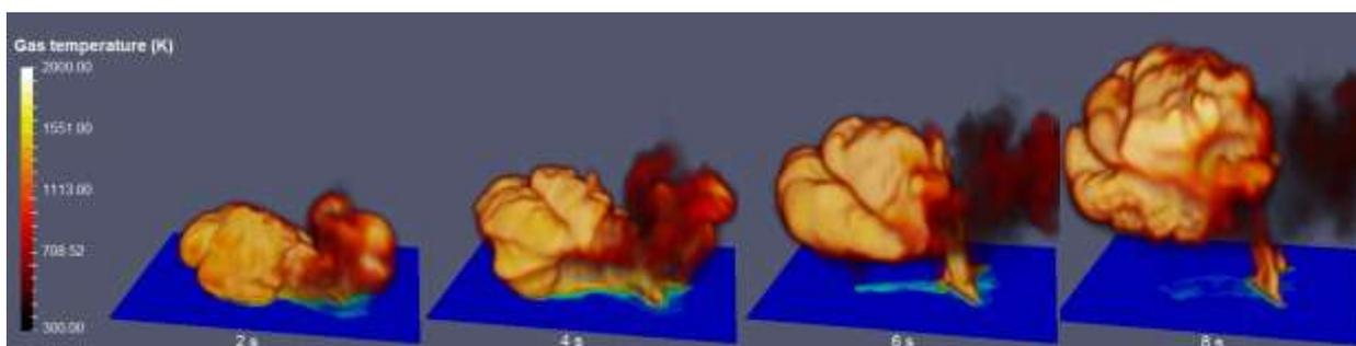
**Figure 7: Fuel spreading with flame (2s), fireball formation (6s) and fireball lifting (8s)**
