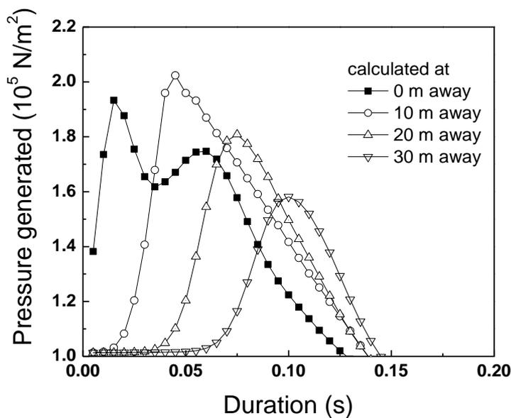
Figure 17: Pressure Calculated in Z direction (0, 10, 20 and 30m)
