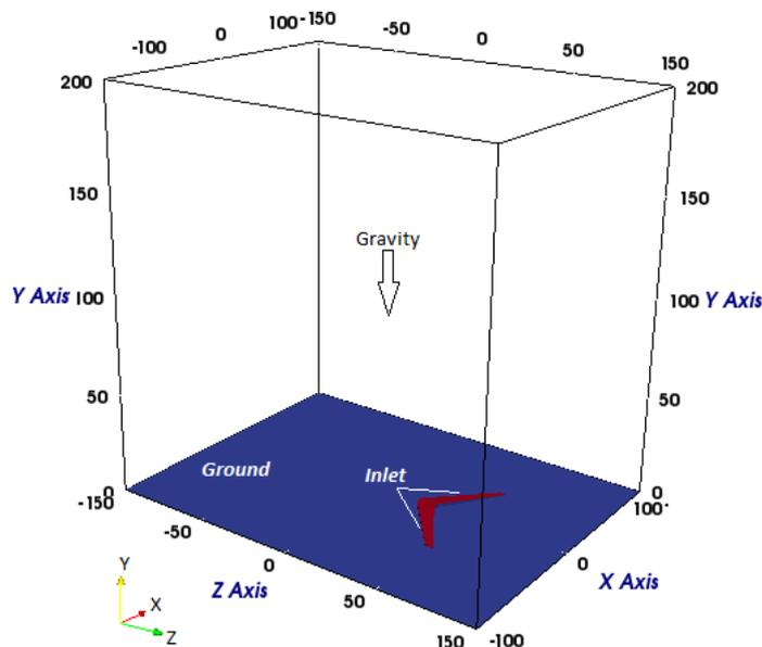
Figure 6: Schematic of computational domain showing the fuel inlet at  $y=0$
