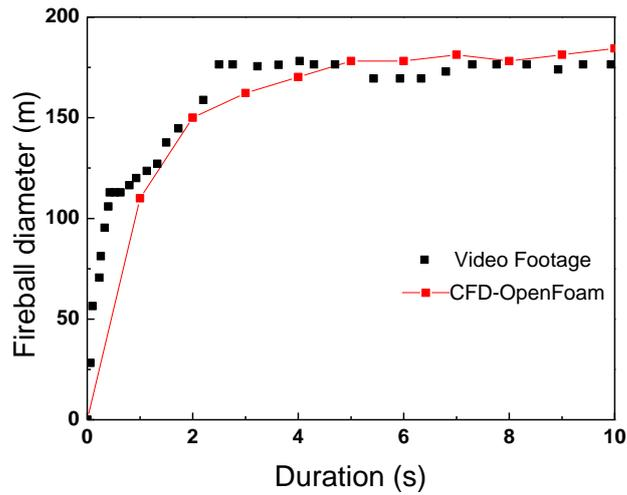
Figure 8: Comparison of fireball diameter from video footage and CFD simulations
