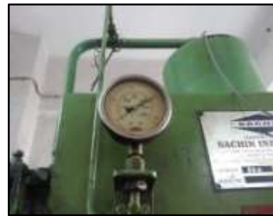
Fig-13: Clamping pressure on moulding machine
