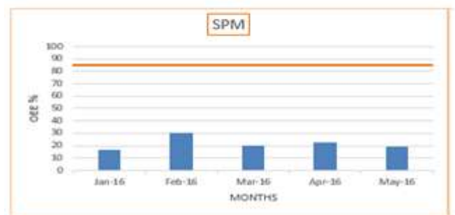
Fig-2: Existed OEE %
