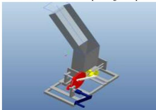
Fig.3.2: 3-D Model (Creo) of Tin Can Crusher
