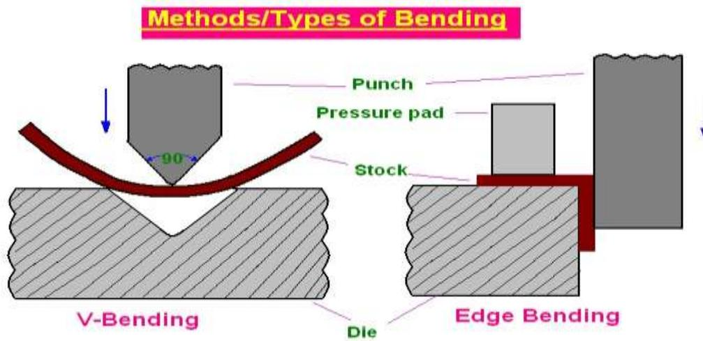
Fig. 4.1: Process bending sheet metal
