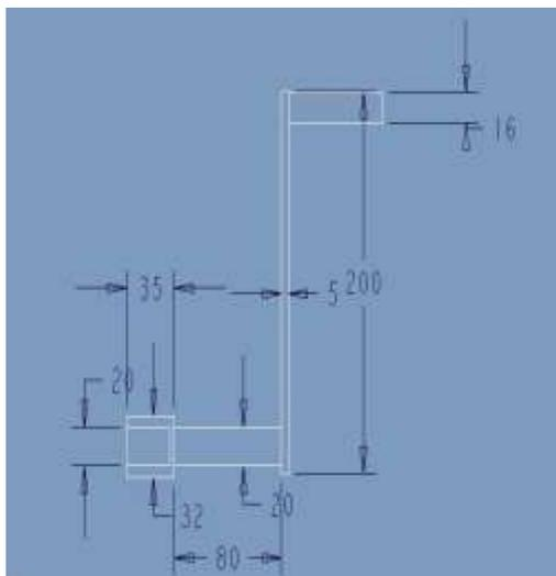
Fig.4.6: Handel and Coupling
