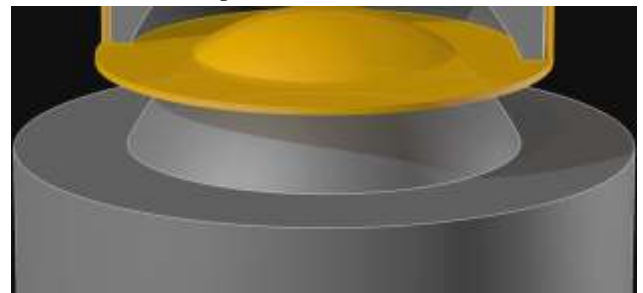
Fig. 9(a) – Doming Tool used to give semi-spherical shape to metal sheet
