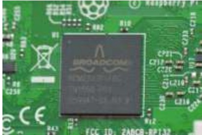
Fig. 4(d) – CPU of Raspberry Pi 3 exposed [19]
