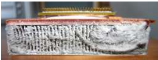
Fig. 7(c) – Dust built-up rendering cooling work offan useless [39]
