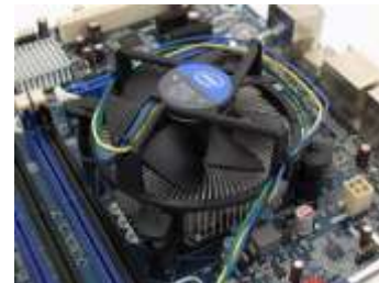
Fig. 4(b) – Active Heatsink cooled by fan [17]
