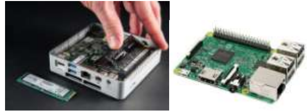
Fig. 2(e) – Mini-PC examples: Intel NUC [11] , Raspberry Pi 3 [12]
