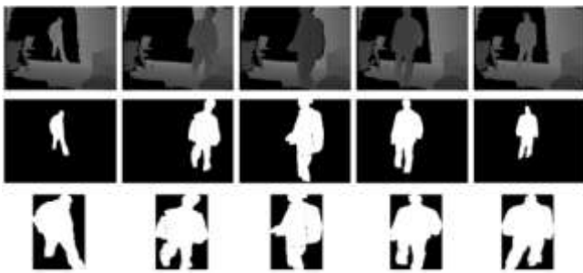
Fig. 1. From top to bottom are the original gait images, binary segmented silhouette images, and normalized and aligned silhouette images of one gait sequence, respectively.
