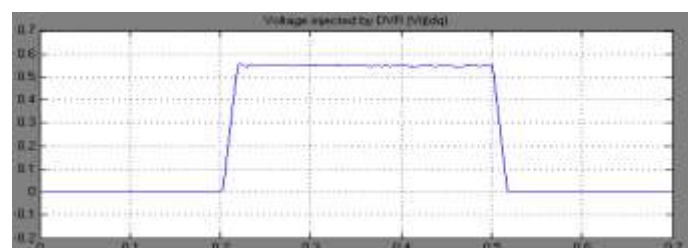
Fig. 9 Voltage submitted by DVR in three phase system
