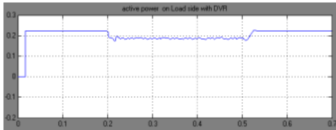
Fig. 13 Active power at load end during compensation
