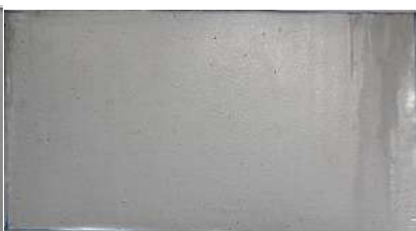
Figure 9: Salt spray test sample nano composite (0.5% ZnO) coated sample after 1200 hrs.
