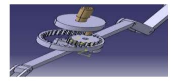
**Fig-3: Internal Gear**
