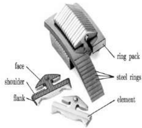
Fig. 3. Composition of Push Belt[8]
